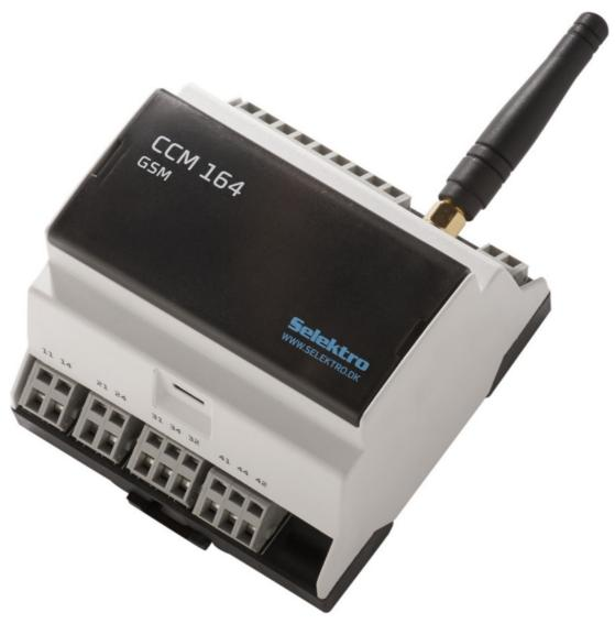
CCM 164 is a control and monitoring module with analog and digital inputs and relay outputs. All inputs and outputs can be monitored and controlled via SMS (Short Message Service) or via a smartphone app. The network is defined by the service provider's SIM card.
